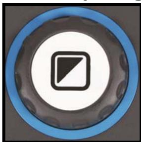
Locate the Zoom dial in the center of the Control Pad. Turn it clockwise to increase the magnification, and counter-clockwise to decrease the magnification.
