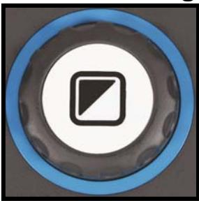
Pressing the white Mode button inside the Zoom dial will cycle you through a maximum of five different viewing modes, depending on how the system is configured:
