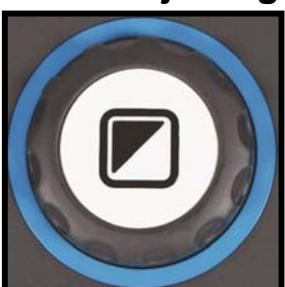
Pressing the white Mode button for four seconds turns off the object lighting. You may want to temporarily turn off the object lighting to eliminate light reflections. If you press this button again, you will continue to the next reading mode and the lights will turn back on. Pressing the button for four seconds will turn the object lighting back on but will not advance to the next reading mode.
