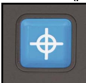
Pressing the blue square Overview button for three seconds will activate a red LED light, which shows as a red spotlight on the reading table. The pointer helps you locate where the camera looks on the table. For instance: when writing, place your pen in the red spotlight on the reading table and the pen will be displayed in the center of your screen. Press this button once again to deactivate the LED light. After 30 seconds, the pointer will automatically be deactivated.
