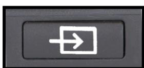
If a computer or another external source is connected to the ClearView C, press the grey PC button marked with an arrow (second button from the right) to toggle between the ClearView C image and the full screen computer image.
